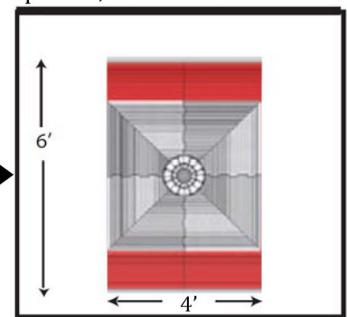
5. Your drain pan is usually precut for this custom drain flange. However if it is not, trim the inside of the pan drain opening to allow for a snug fit of the flange. It should fit as seen in the picture (this example shown in a 32x60 pan) and the drain outlet on the bottom side of the pan should look like the second picture.
