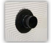
6. Test Fit drain flange in pan and measure distance to 2" waste pipe fitting under subfloor. Cut and test the proper length coupler pipe that will attach flange to waste pipe but still properly seat flange into pan/floor assembly. Ensure that this is correctyour next step will be to glue the flange to the waste pipe plumbing.
